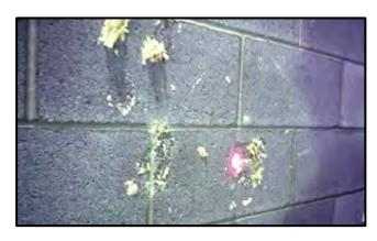
Tests have demonstrated excellent resistance to impacts of wind-borne objects. Projectiles that penetrate stud-based walls are stopped by solid grouted concrete masonry walls.
